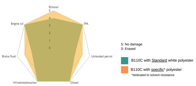
These performances are for guidance only. Results are obtained with adapted receiving material and optimum print conditions. (Ricoh test method)
