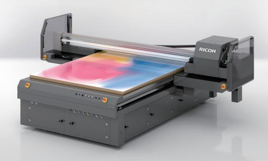
The new RICOH Pro T7210 UV Flatbed combines impressive print speed and excellent image quality. Built for productivity with customization capability and material versatility. The integrated vacuum table with pin registration makes handling and positioning of materials easy. Full bleed printing eliminates the need for trimming or cutting hence, reduce the finishing time.
