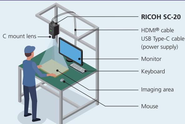
\* A mouse and keyboard are not necessary when using a touch panel monitor.
