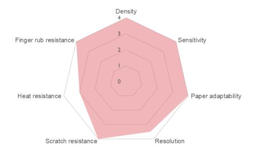
These performances are for guidance only. Results are obtained with adapted receiving material and optimum print conditions. (Ricoh test method)
